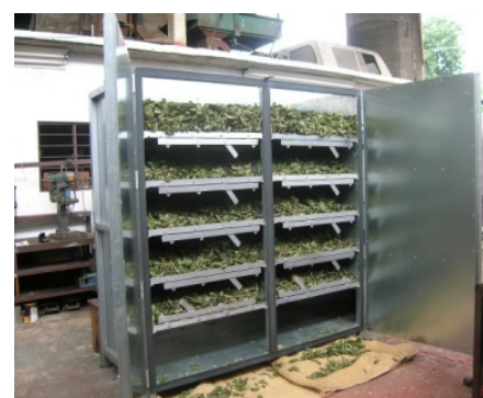
Prototype machinery for drying guava leaves
